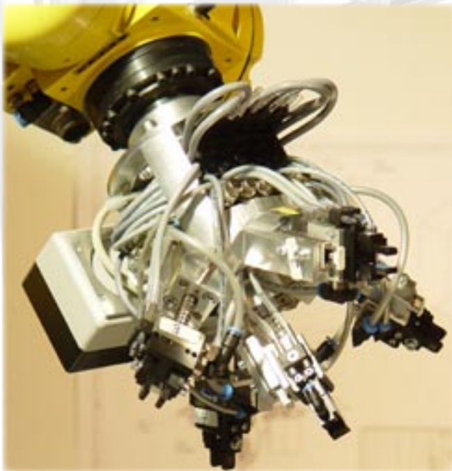
Example: 5-gripper robot tool 8 outputs, 16 inputs
